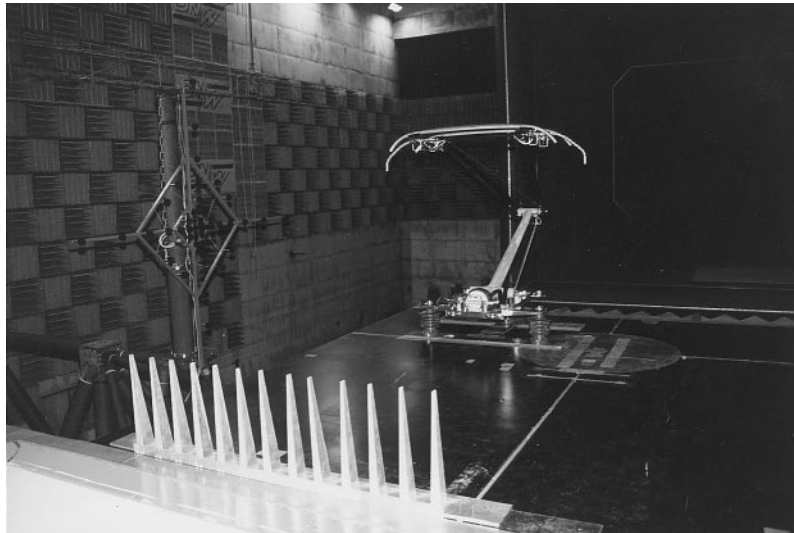
Figure 20. Overview of experimental set-up showing pantograph (middle), acoustic antenna (left) and vortex generators (front).
